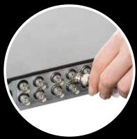
Connect the 8-way power splitter to each of the extension cable power plugs.
