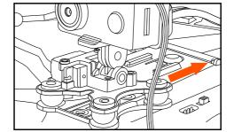
d. Plug both data cables into the corresponding plugs near the Skyview HD Quadcopter's on/off switch
