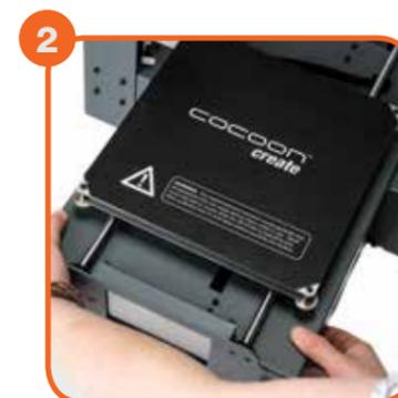
Insert the Heated Print Bed Controller carefully through the legs of the Extruder Tower and align the bolt holes on each side. Using the Hex Wrench, insert and tighten the two bolts on the bottom of each Extruder Tower
