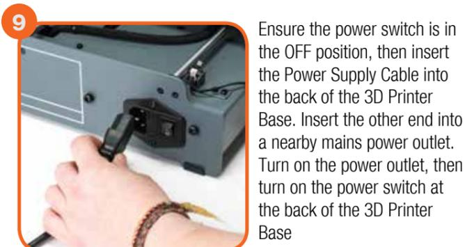
Ensure the power switch is in the OFF position, then insert the Power Supply Cable into the back of the 3D Printer Base. Insert the other end into a nearby mains power outlet. Turn on the power outlet, then turn on the power switch at the back of the 3D Printer Base
