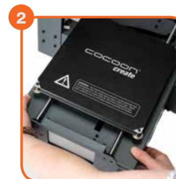
2 Insert the Heated Print Bed Controller carefully through the legs of the Extruder Tower and align the bolt holes on each side. Using the Hex Wrench, insert and tighten the two bolts on the bottom of each Extruder Tower
