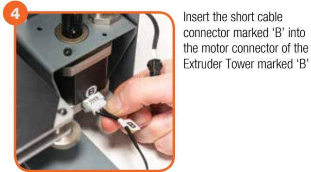
Insert the short cable connector marked 'B' into the motor connector of the Extruder Tower marked 'B'
