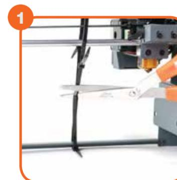
1 Place the Extruder Tower and Heated Print Bed on a clean, level work space. Carefully remove the cable tie that holds the extruder in place.
