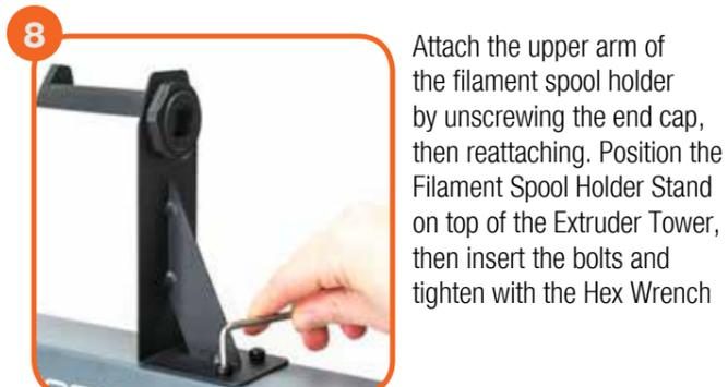
Attach the upper arm of the filament spool holder by unscrewing the end cap, then reattaching. Position the Filament Spool Holder Stand on top of the Extruder Tower, then insert the bolts and tighten with the Hex Wrench
