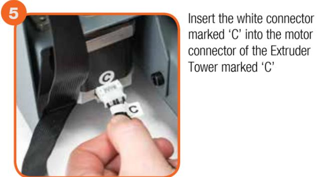
Insert the white connector marked 'C' into the motor connector of the Extruder Tower marked 'C'
