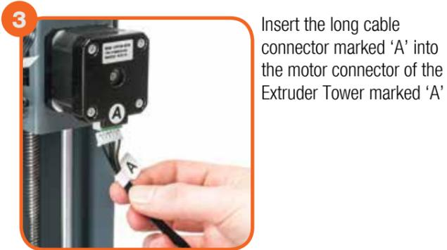
Insert the long cable connector marked 'A' into the motor connector of the Extruder Tower marked 'A'
