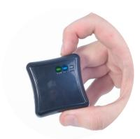
REGISTER YOUR MOBILE SMS 123456A1 to the phone number of the SIM card used in the Cocoon GPS tracker.
