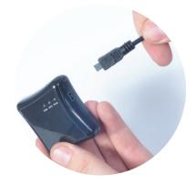
HOLD DOWN POWER BUTTON Hold the power button for 5 secs then release. The unit is powered on when the GSM & GPS buttons are illuminated.
