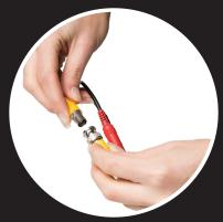
Connect the other end of the extension cables to the ports marked "Video IN" on the back of the DVR.
