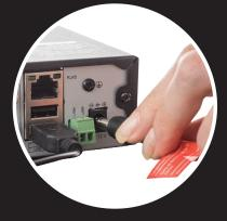
**Tips**: Test all connections are working before permanently installing DVR and cameras. Position the DVR in a central location where all 8 cameras will reach. If using the optional networking features make sure the modem is near the DVR
