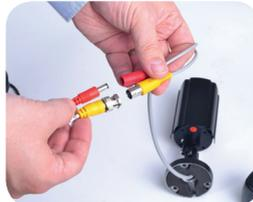
2. Connect the other end of the extension cables to the video cable splitter, and then connect the cable splitter to the port marked "Video Input 1-4"
