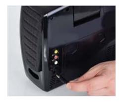
**CONNECT YOUR MICROPHONE** Connect the included microphone to the port marked MIC 1 on the front of the unit.
