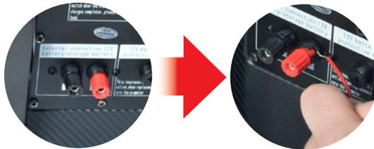
2. Once the wire has made contact behind the battery connector point, tighten the screws to ensure the wires stay in place.
