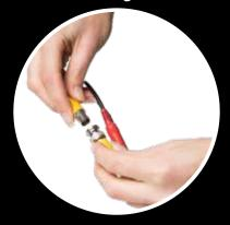
Connect the other end of the BNC extension cables to the video cable splitter. Connect the splitter to the port marked "VIDEO IN/OUT" on the side of the DVR.
