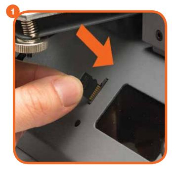
Insert the included MicroSD Card into the memory card slot next to the LCD screen with the label facing to the left as shown
