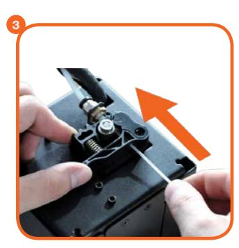
After the extruder has fully preheated, hold the filament clamp on the top of the tower and manually feed the end of the filament through the tube until you feel some resistance. Let go of the clamp so the motor can push the filament through
