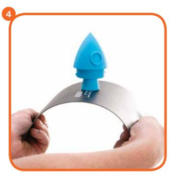
Once the print is complete, turn off your 3D Printer and wait for the extruder to cool. After removing the magnetic print mat from the printer base, slowly and gently bend the sides of the mat down to raise the center of the mat and lift the printed object
