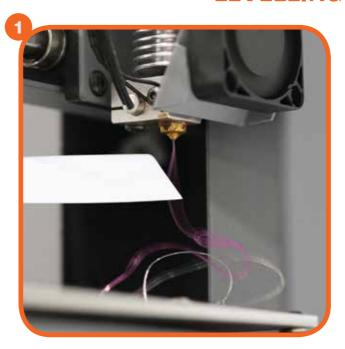
Clean off any excess filament residue from the tip of the nozzle using the scraper
