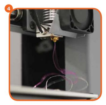
Once filament is extruding from the nozzle press back to stop extruding
