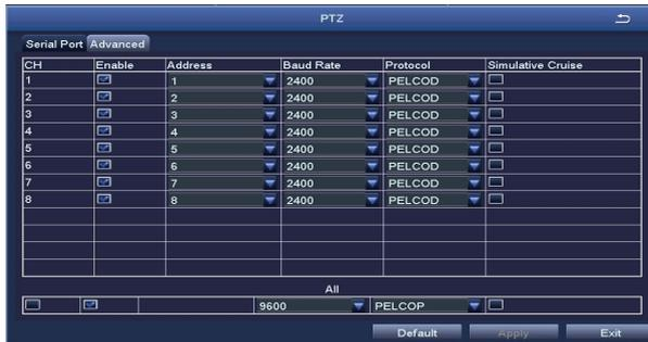
This DVR unit is compatible with PTZ (Pan, Tilt & Zoom) cameras (not included). Access this page to configure the PTZ camera settings. Please note that the PTZ device can be activated only when a channel in connection with the PTZ camera is selected. Consult the manual of your PTZ camera for correct settings.
