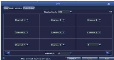
**NOTE:** If 1x1, 2x2 or 3x3 is used, Start/Stop Scan can be used on the viewing screen to automatically change between cameras.
