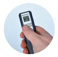
**TURN OFF** Turn off the device by holding down the PLAY button for 2 seconds
