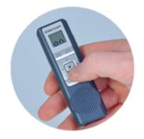
**RECORDING** Press the REC button once. The record icon REC will be shown on the LCD display
