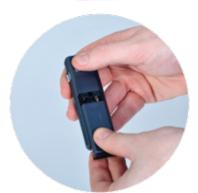
**INSERT BATTERIES** Insert the supplied 2 x AAA batteries according to the marked polarity. Replace the battery cover
