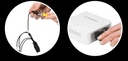
**3.** Connect the 4-way power splitter to each of the extension cable power plugs.
