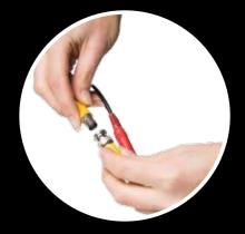
2. Connect the other end of the extension cables to the video cable splitter. Connect the splitter to the port marked "VIDEO IN/OUT" on the side of the DVR.
