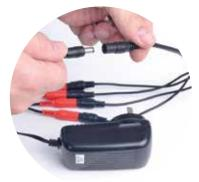
Connect the remaining power adaptor to the DVR and plug into a mains outlet. Switch the outlet on. The DVR will begin the boot sequence.
