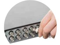
**3.** Connect the 8-way power splitter to each of the extension cable power plugs.
