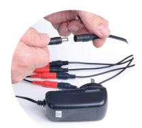
**7** Connect the remaining power adaptor to the DVR and plug into a mains outlet. Switch the outlet on. The DVR will begin the boot sequence.
