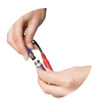
2. Connect the other end of the extension cables to the ports marked "VIDEO IN" on the back of the DVR
